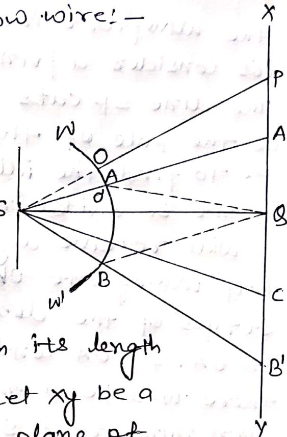
Let SA and SB produced meet the screen XY in A' and B'. Then A'B' is the region of the geometrical shadow of the wire. According to rectilinear propagation of light, there should be uniform illumination above A' and below B', and complete darkness within A'B'. But actually, unequally-spaced bands with poor contrast and running parallel to the length of the slit are observed in the region above A'
